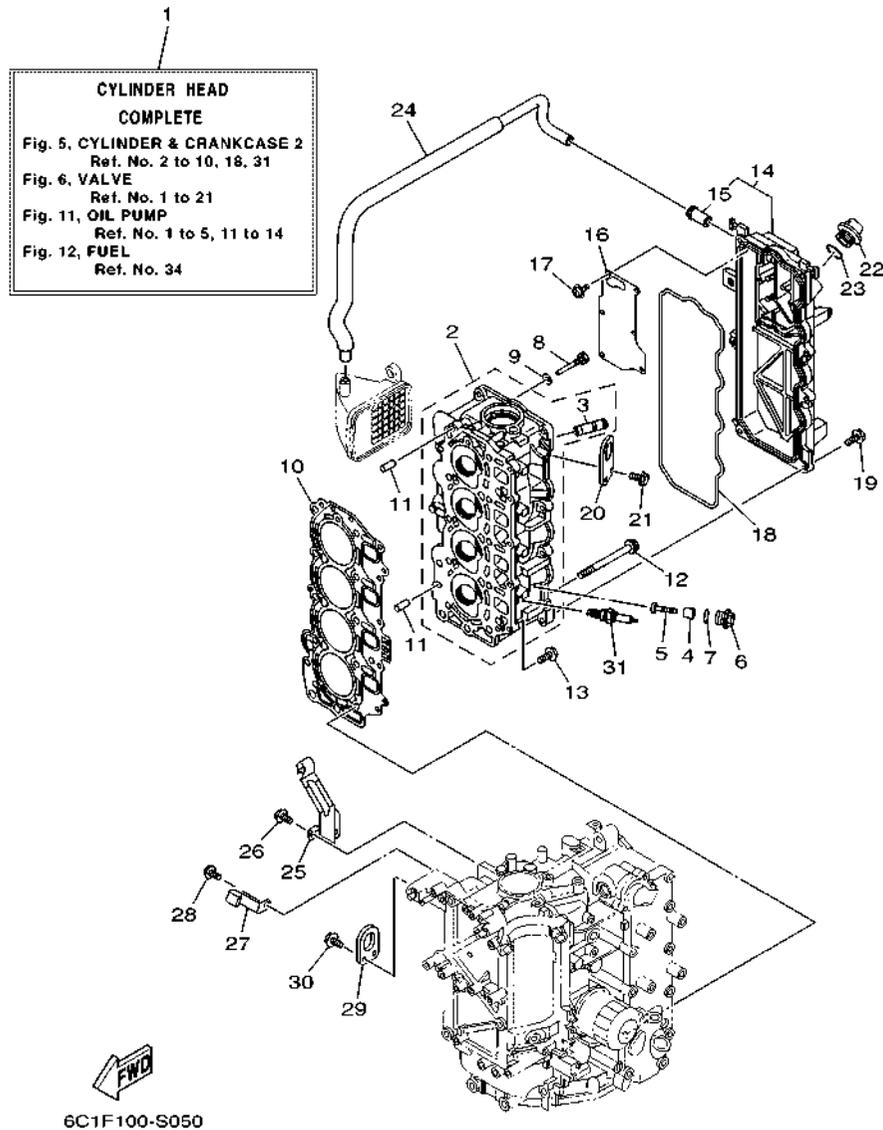
FIG. 5 CYLINDER & CRANKCASE 2
