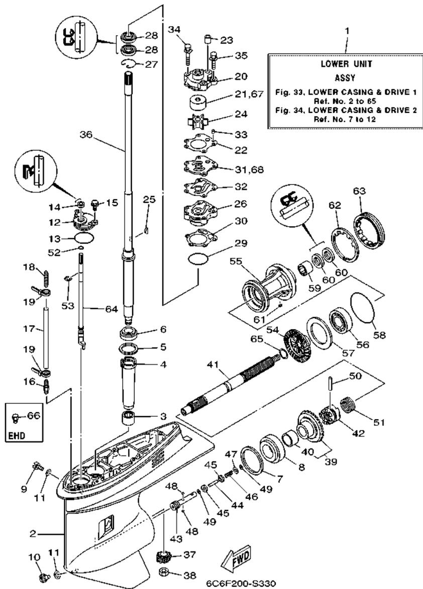
FIG. 33 LOWER CASING & DRIVE 1
